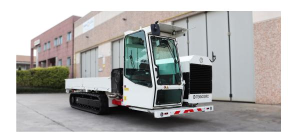
The machine is equipped with Gemmo Group crawler undercarriage and Cummins B4.5 Stage V - Tier 4F 149 kW - 780Nm engine.
