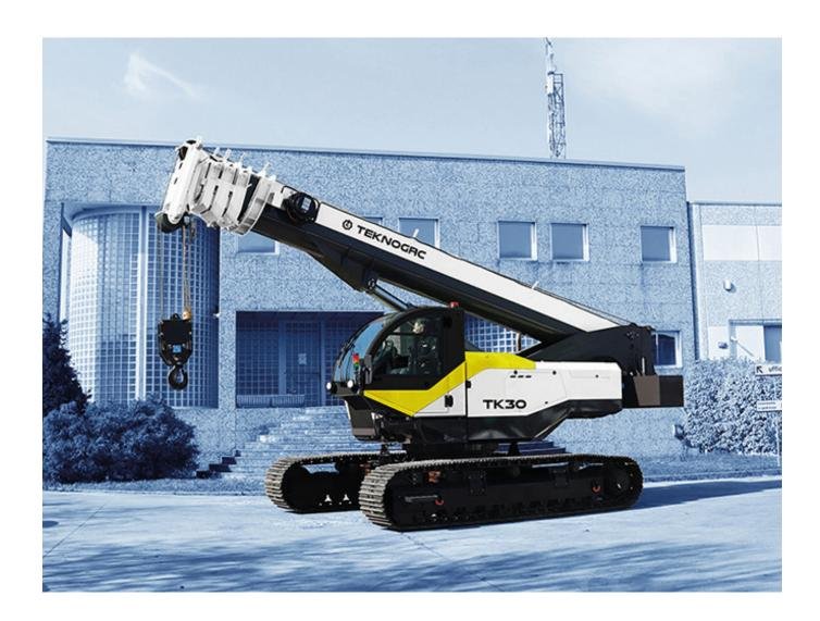
The TK30 is a compact and easy to maneuver crawler crane. Its steering wheel, its translation system managed by a Danfoss control unit and its small size allow the operator to maneuver this crane in restricted areas. The tracked undercarriage with widenable track and the height of only 3015mm guarantee ease of loading and transport.
