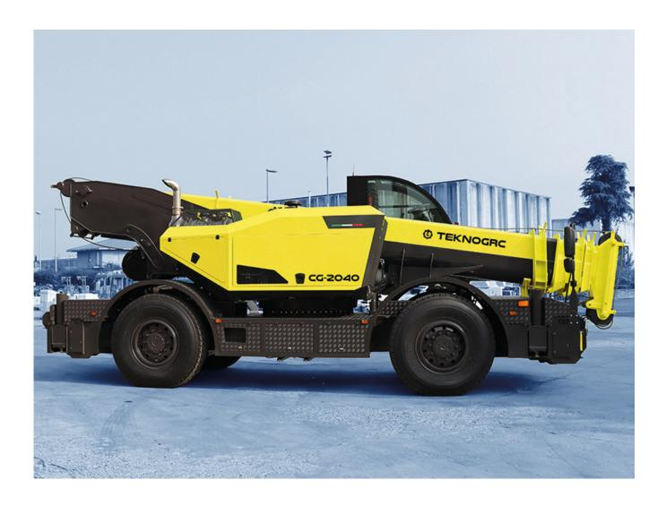
The CG-2040 is a compact and powerful mobile crane suitable for different working conditions. The innovative fully adjustable horizontal suspension system, the result of 40 years of experience in the lifting field, allows the most impassable workplaces to be reached. The small dimensions make the CG-2040 the ideal vehicle for lifting and handling operations even in city contexts. The attention to the environment and the low level of emissions allow the free movement of the crane.
